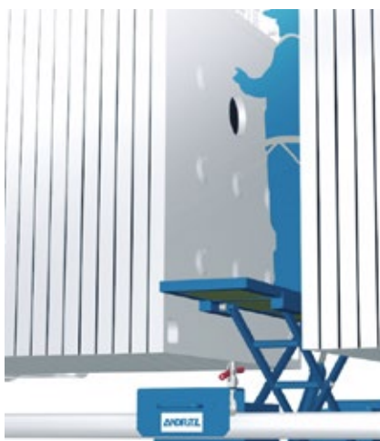
SmartLIFT for easier, safe, and faster exchange of filter cloths for overhead filter presses
