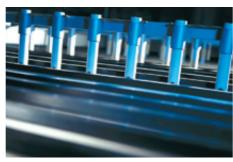
Efficient drainage rolls to minimize rewetting
