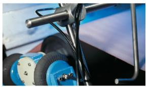
Optional: Wire tensioning via air cylinders
