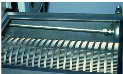
Sieving basket and wash water pipe in the U-trough.
